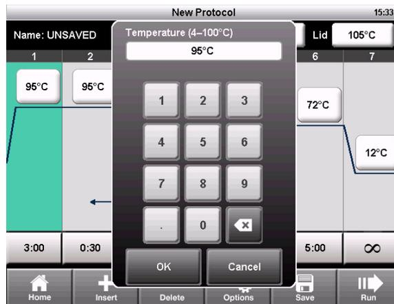
**Figure 7. Editing a temperature with the numeric keypad.**
