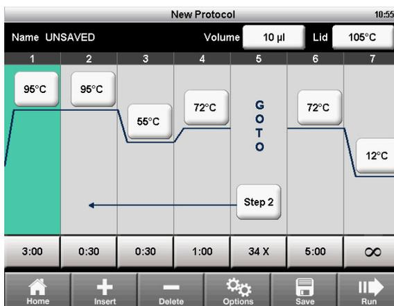
**Figure 6. The template for a PCR protocol.**
