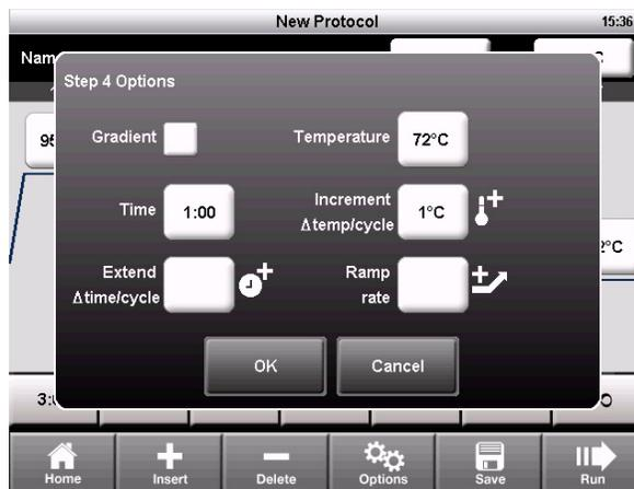
Figure 12. Step 4 has a temperature increment option.
