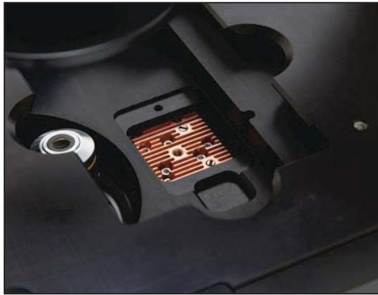
Loosen slotted screws with tool
