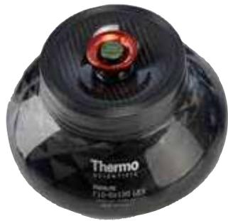
**Fiberlite F10-6x100 LEX 碳纤维角转头, 45°, R<sub>max</sub> 122 mm**
